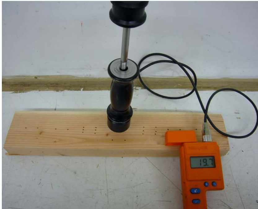
Figure 2. Moisture measurement with digital moisture meter.
