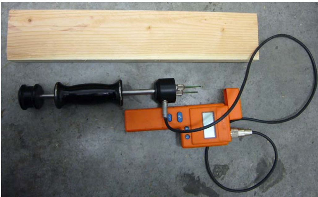
Figure 1. Delmhorst J-2000 digital moisture meter and 18-inch 2 X 4 section of main fuel load.
