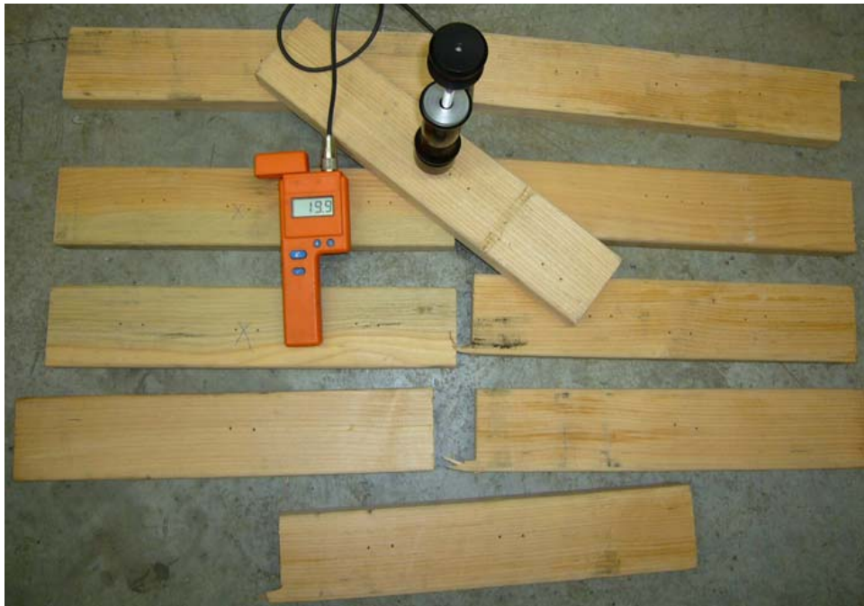
Figure 4. Moisture meter measurements made on 10 2 X 4 pieces cut from a single 4 X 4.
